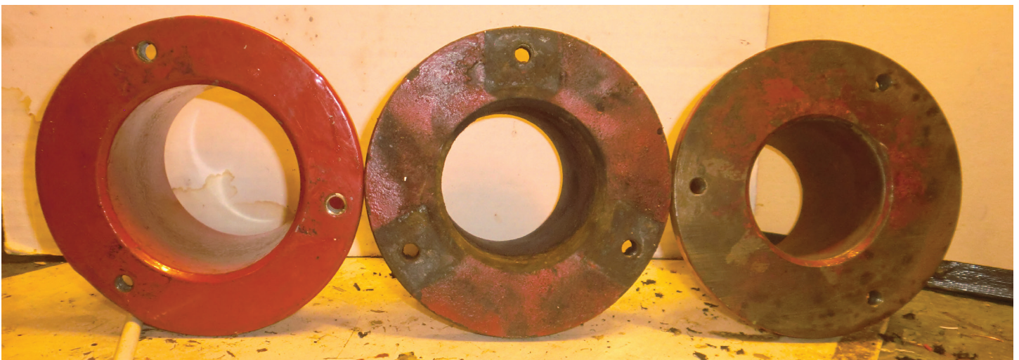
Figure 3: (ref file 6250) Back side of figure 1. 4", 3.5" and 3.25". Note the chamfer on each pulley, regardless of size.
