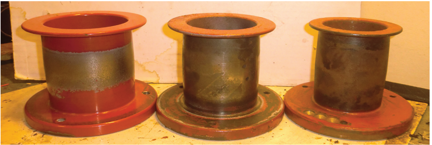
Figure 2: Left to right: 4" Standard, 3.5" and 3.25" pulleys. Note the curved pulling face on all pulleys, needed to keep the belt centered. All photos by the author.
