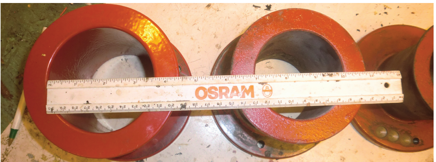
Figure 4: Measurements showing center hole diameter is 0.5" less than outer pulling face diameter. Left pulley is standard 4" pulley (shows 3.5" inside diameter), right is 3.5" pulley which shows a 3" inside diameter).
