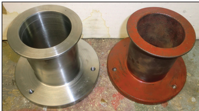
Figure 1 Above: Machined copy (left) next to original Fairmont 3.25" factory pulley (right). All photos by the author.
